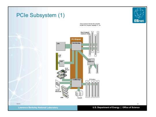
The Chipset is the component in the server that handles all the I/O. In other words, it is responsible for moving data from the PCI cards and the CPU.
