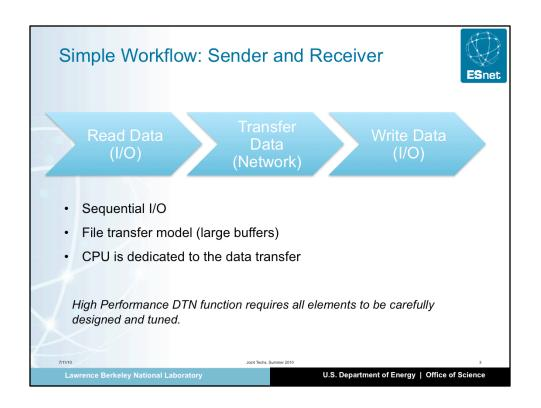
A Data Transfer Node is not a processing, rendering, server. Its only workflow is:
