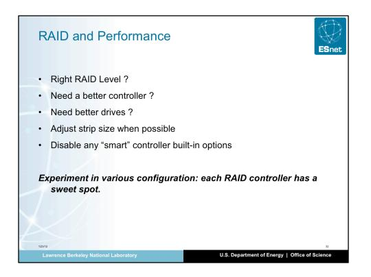
Disk controllers, RAID or not, are usually designed for "entreprise". This usually means that the controller is often configured with RAID 5 or 6. As a consequence, controller are most of the times, not capable of running all the drives at full speed: in entreprise context, there are always a few drives that are hot replacement. A rule of thumb is that if a controller is said to handle up to X drives, it can handle up to 2X/3 drivers at full speed.
