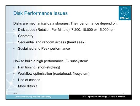
Designing a RAID system is almost an art: there are so many constraints that while it is almost always possible to optimize the storage subsystem, it is almost always impossible to get what you really want. When working on the storage subsystem, ask yourself the following questions:
