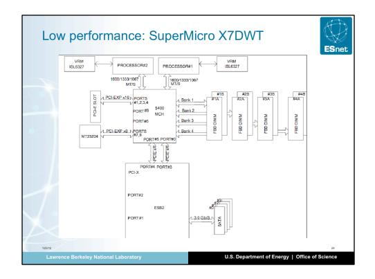
This is not a bad motherboard, just not designed for performance. It has only one chipset (but still two processors). It also has a single memory bank.
