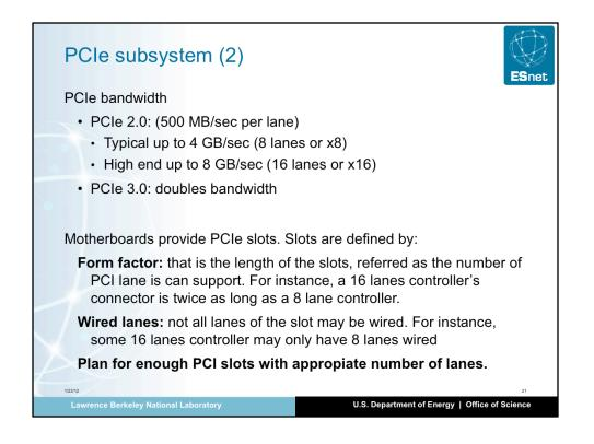
In order for the overall system to performance to the specifications, it is critical to set the card into the appropriate slot:
