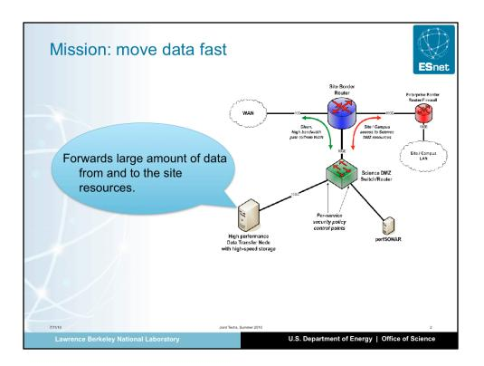
A Data Transfer Node has only one mission to fulfill: send large amount of data across thousands of mile as quickly as possible.
