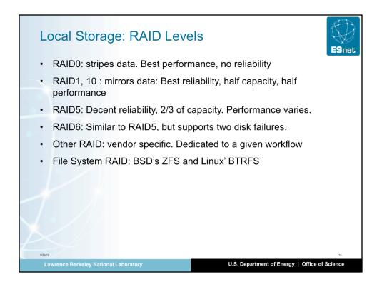
RAID0 is the right choice when try to get the maximum storage performance at the lowest cost (the lowest number of drives). A single drive failure will cause the entire volume to be lost.
