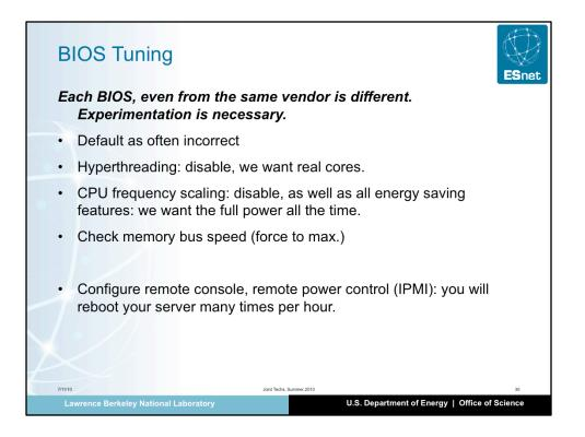
BIOS tuning can be painful. A wrong setting can have dramatic effect on performance, but also on stability of the system. The goal is to make the behavior of the hardware as predictable as possible and to run it at maximum performance.
