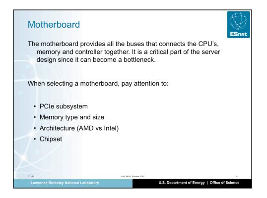
The motherboard not only incorporates the CPU's and memory, it is also providing all the busses between the various component of the server. An inadequate motherboard can become a major bottleneck. It is, then, very important to correctly select it. The questions to ask while selecting are:
