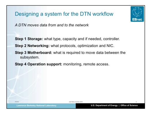
In a nutshell, the motherboards moves data from/to the storage to/from the network. It is critical that this can be accomplished efficiently.
