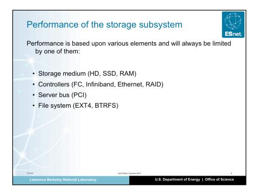
Performance of a storage subsystem varies depending on its type and architecture.
